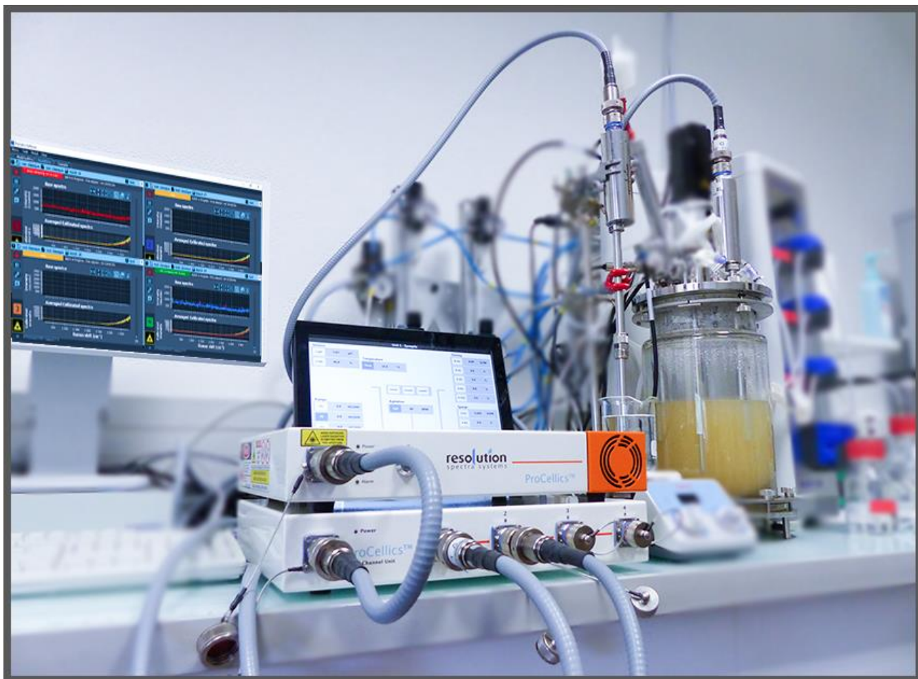
Images: ProCellics™ In-Line and Real-Time Bioprocess Raman Analyzer Multi-Channel Unit and ProCellics™ Software
